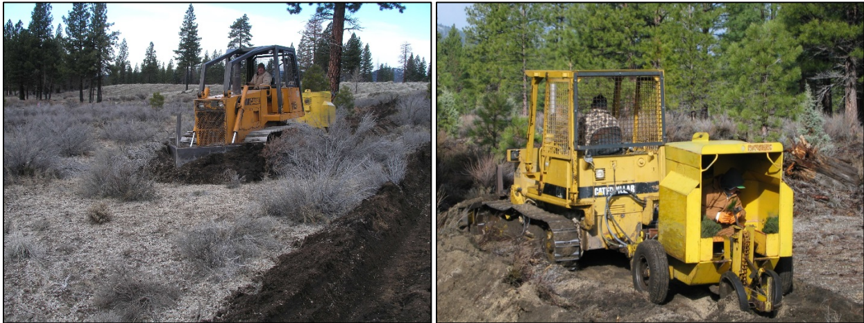
Figure 9.12 A “V Blade” attached to the front of a crawler tractor scalps away grass and brush making a level surface of moist mineral soil (left) in preparation for planting 2-0 bareroot ponderosa pine seedlings by the planting machine attached behind the crawler tractor.
